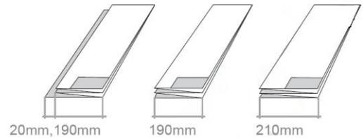
**Cross folding:** 297 mm or 305 mm obtained by re-introduction of fan folded document. Automatic detention of one or two cross folds.
